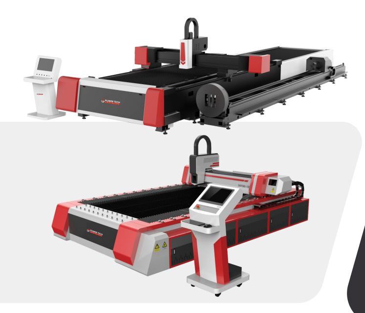
The focussed laser beam is directed at the material, which then either melts, burns, vaporizes away, or is blown away by a jet of gas, leaving an edge with a high-quality surface finish.
